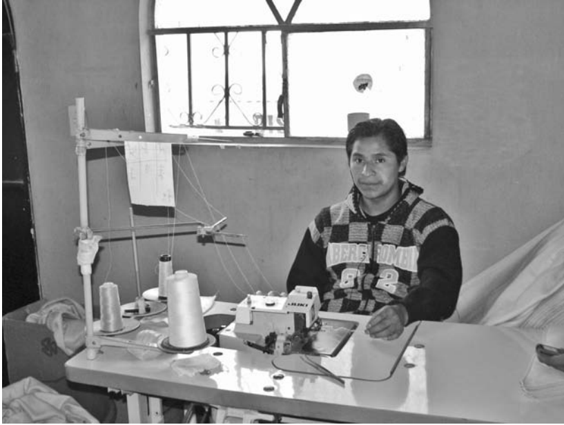
FIGURE 8. Teenage workshop employee seated at a serger machine, which is used to finish the edges and seams of knit fabric, Tecpán, 2009. Note that he is wearing a knockoff Abercrombie & Fitch sweater.
