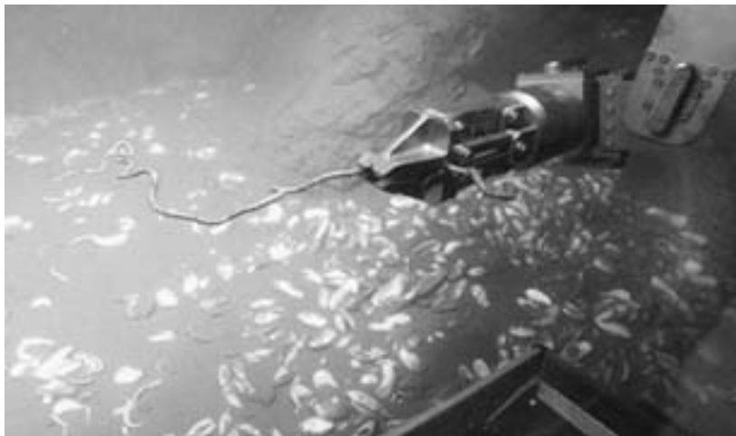
FIGURE 7. VICKI frame grab of Ventana's vantage point as the ROV arm grasps a tubeworm. ©2003 MBARI. Reproduced with permission.
